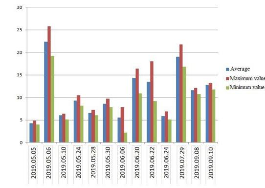
In 2019, no significant difference could be observed during major precipitation events, as was the case more often in 2018. During the 13 days, the value of the standard deviation exceeded the value of 2 mm only once with its value of 2.77 mm on 22.06.2019, with an average of 13 mm/day.
